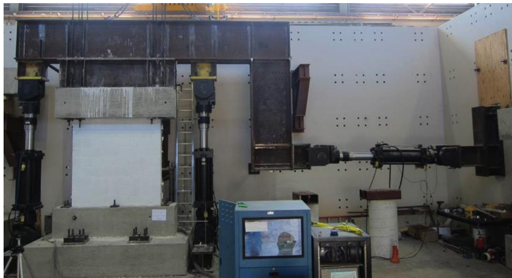
Figure 3.5 - Test setup for wall UT-PBS-01 (Ahmadi, 2012)
