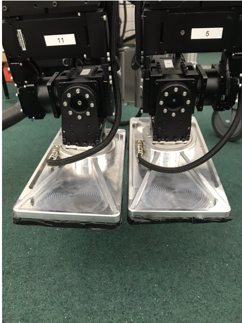
Figure 2.12: PEBL's redesigned, slimmer feet. The original feet barely avoided collision when the THOR-OP was in its home position.
