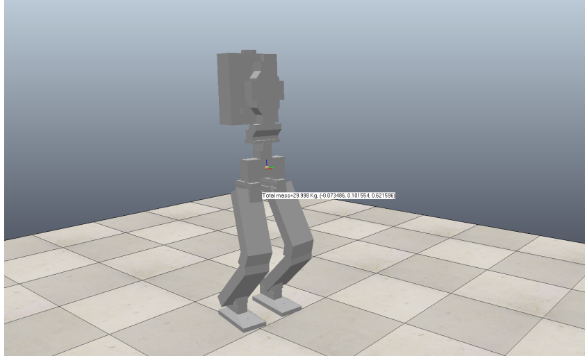
Figure 2.18: Dynamic simulation of PEBL walking using CoppeliaSim.
