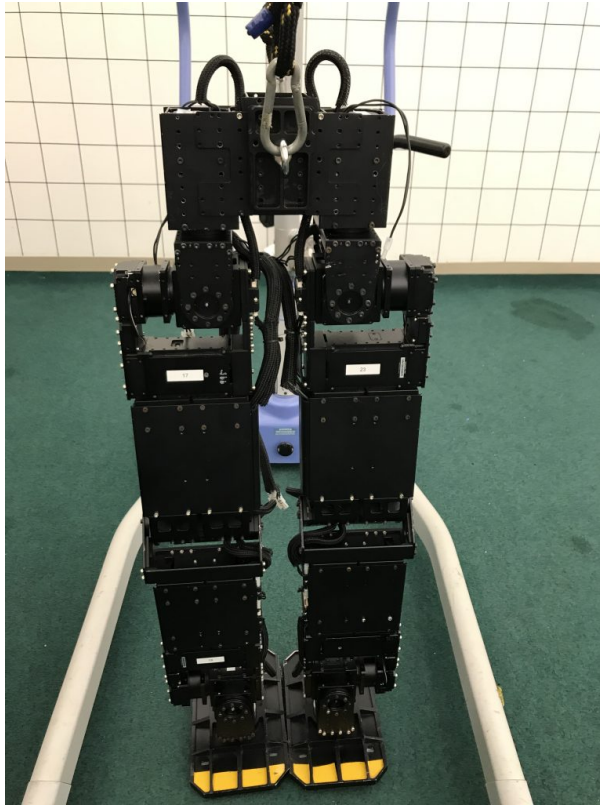
Figure 2.3: PEBL1, lower body of THOR-OP, with offboard computing and no sensors.
