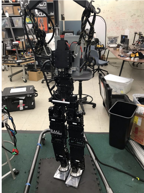
Figure 2.5: PEBL3, with new F/T sensors and torso which shifted the center of mass higher.
