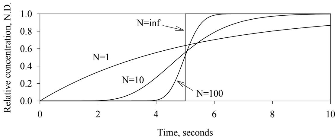
**Figure 2: Approximation of plug flow by mixing systems.**
