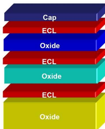
Figure 5.4: Schematic diagram of the ECC media. Between the cap layer and the granular layers (oxide layers) there are the exchange-coupled layers.
