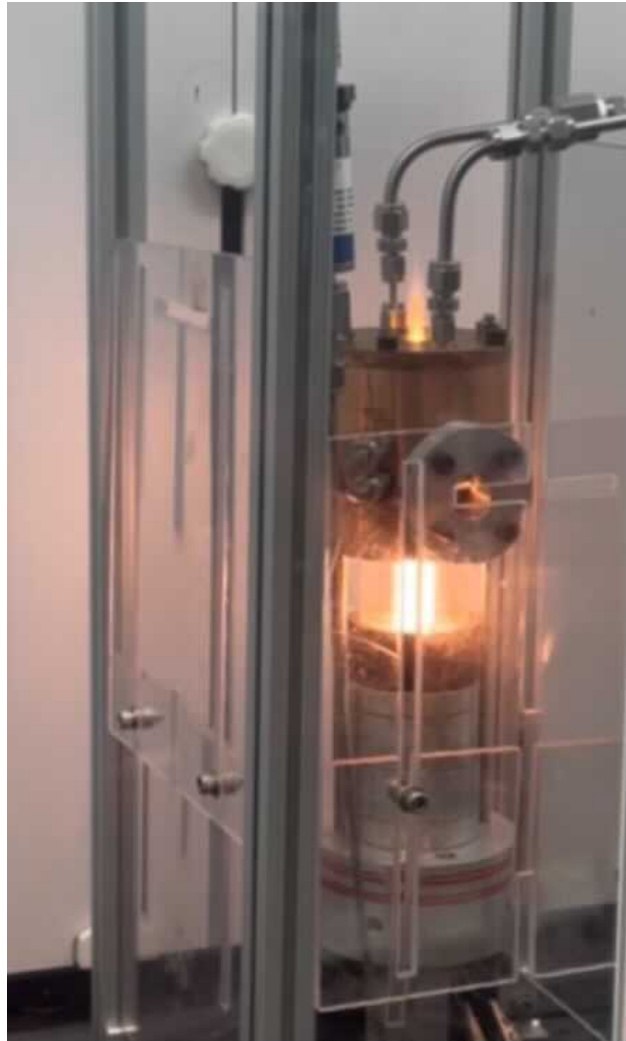
Figure F.2 High pressure hybrid rocket test rig during a hot fire test with P_c = 10\text{bar} .
