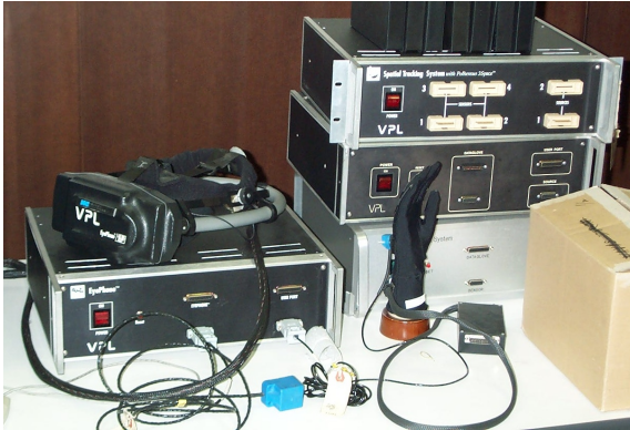
Figure 4.7: EyePhone HMD and Data-Glove by VPL [Pap]
