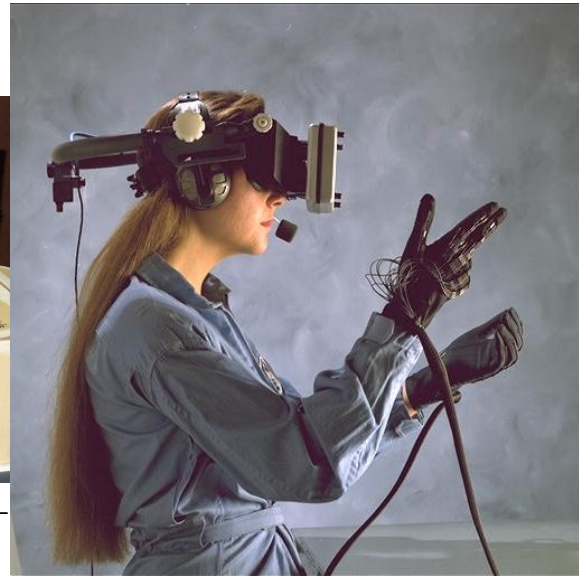
Figure 4.8: HMD and Wired Gloves - Ames Research Center [NAS06]
