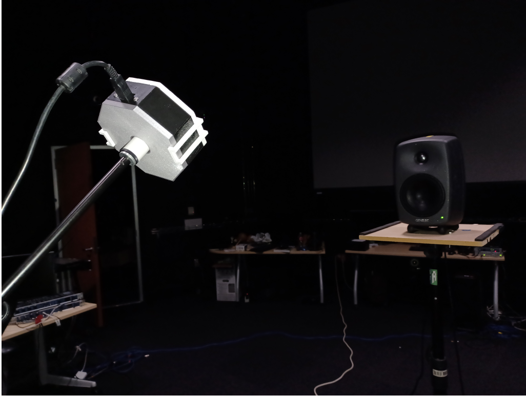
Figure 3.9: The microphone Measured for 3OA SHs (45 degrees)
