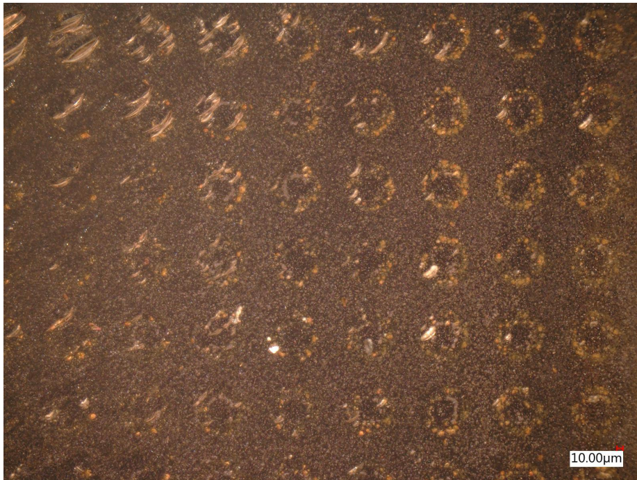
Fig. 4.19 Microstructure of non-bonded die on the top wafer post reflow at 300x
