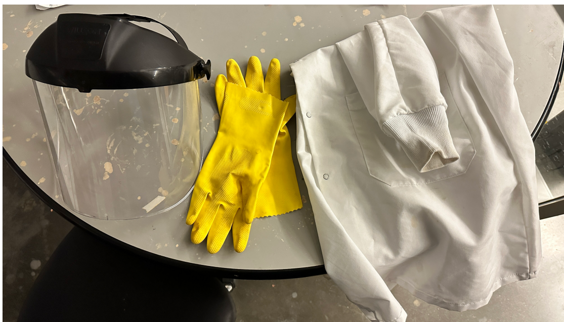
Fig. 2.6 Necessary safety measures for performing the electroplating process
