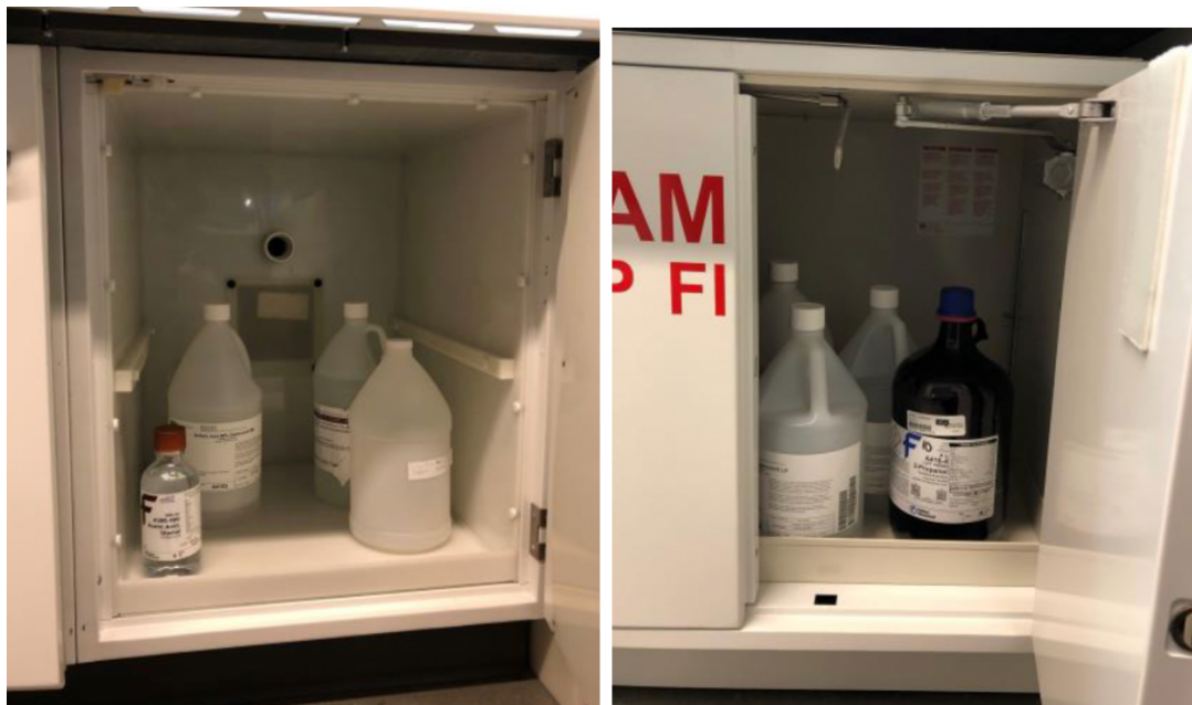
Fig. 2.7 Acid bottles go in the plastic cabinet (left) and organic bottles stored in steel (right) [9]
