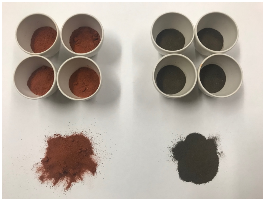
Figure 4.1 Picture of an exemplary set of mineral soil (left) and autoclaved soil (right) samples used in this study. The reddish-brown color of the mineral soil indicated the majority organic matters were depleted after the “Loss on Ignition” combustion process.
