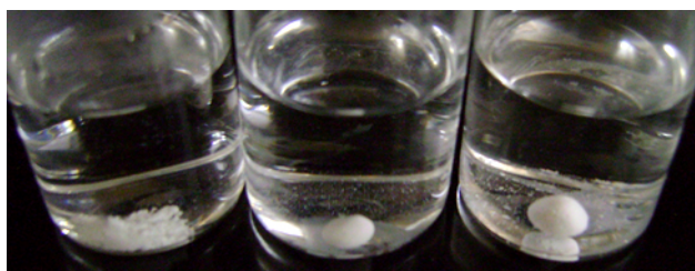
Figure 3-11. Washout test on ELP-CPC composites. After mixing, cements were immediately immersed in 37 °C HEPES buffer. CPCs without ELP (left) were unstable and disintegrated while the E8-ELP containing mixtures remained as cohesive masses.
