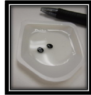
Figure 2 - India Ink measured in a pool of silicone
