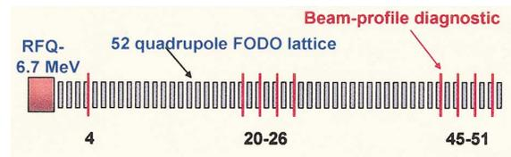
FIG. 1 (color). Block diagram of the 52-quadrupole-magnet lattice showing the nine locations of beam-profile scanners.
