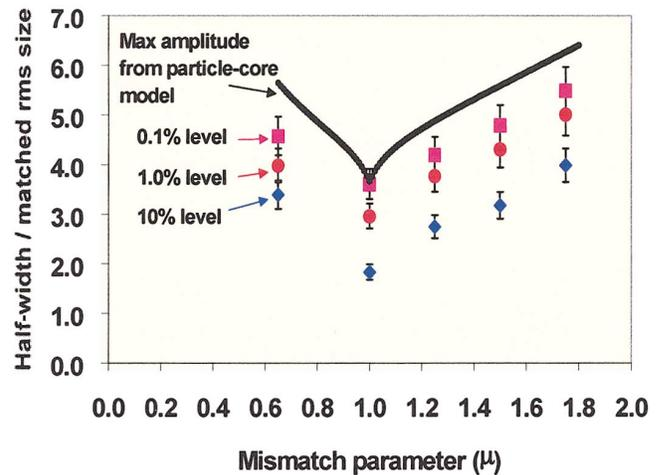
FIG. 5 (color). Measured beam half-widths at scanner 20 (75 mA and a breathing-mode mismatch) at different fractional intensity levels versus mismatch strength  $\mu$  for comparison with the maximum resonant amplitude of the particle-core model. Equation (6) of Ref. [5] gives an approximate expression for the theory.
