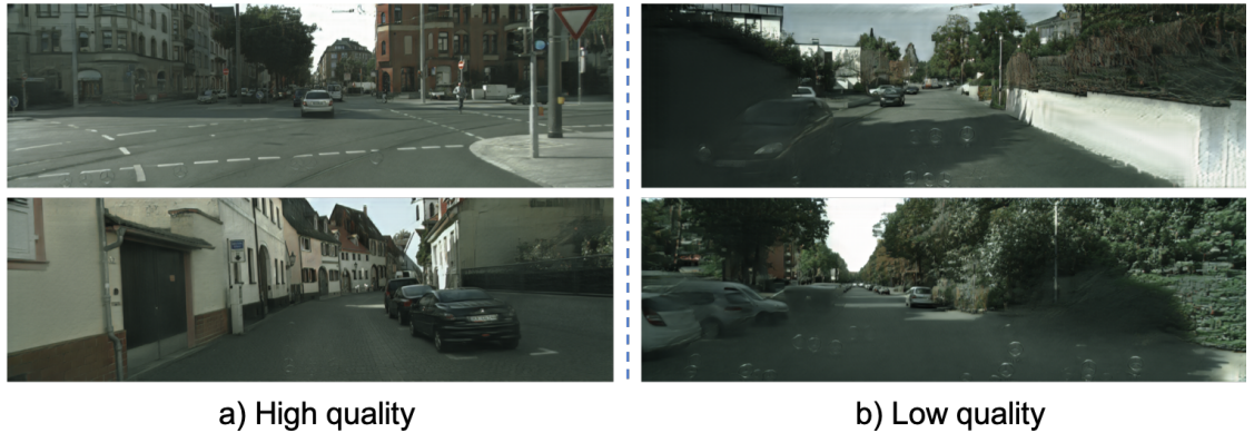
Figure 4.5: Image quality examples from the KITTI dataset synthesized to be in the Cityscapes domain. a) shows the ones that are translated with better quality. Images in b) contain artifacts and fail to preserve details of the car, almost blending into the background.
