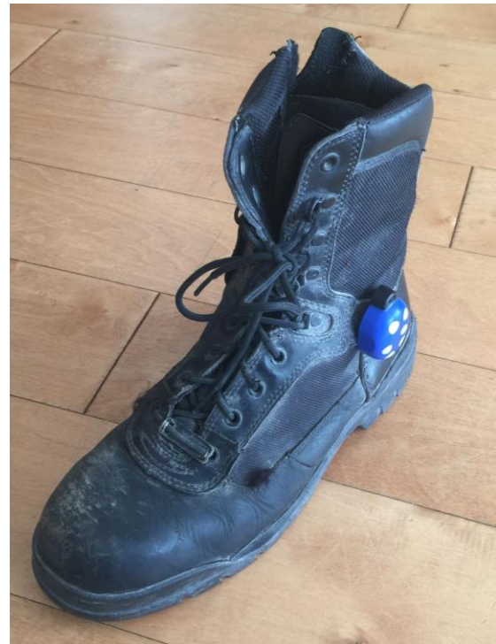
Figure 4 Mounting of the SmartBug IMU for Pedestrian Navigation
