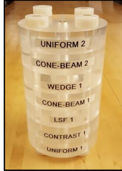
FIG 3.4. Photos of the (a) Defrise phantom and the (b) Corgi phantom used in the quantitative experimental study. (c) Line pair demonstration to show the calculation of the loss in modulation in the z -dimension ( z_{mod} ) through the volume data set of the Corgi phantom cone beam artifact module.
