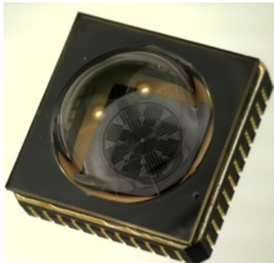
Figure 4.27: 50 mm 3 3D MEMS IMU in an LCC standard package with a “bubble-shell” glass lid.
