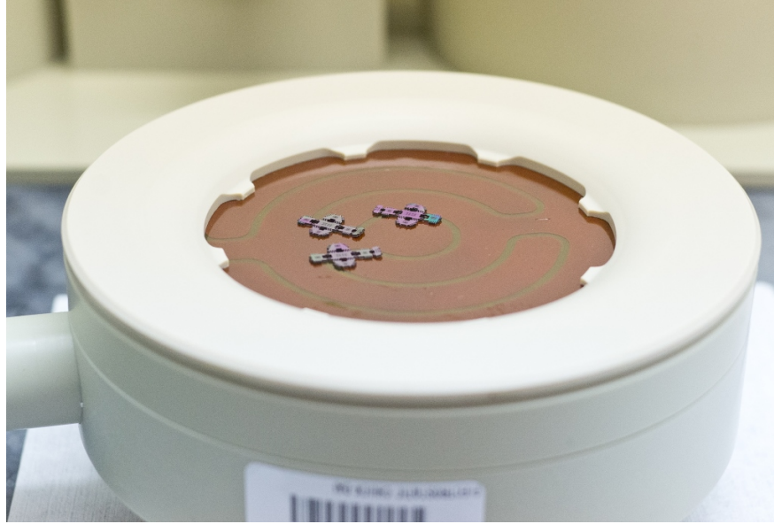
Figure 3.19: Unfolded IMU structures are placed on the electrostatic chuck of the IDONUS HF Vapor Phase Etcher.
