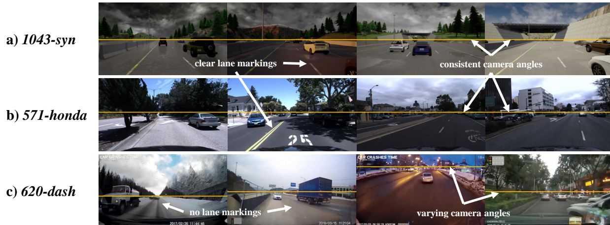
Figure 4.9: Examples of driving scenes from our a) synthetic datasets, b) typical real-world dataset, and c) complex real-world dataset. In a), all driving scenes occur on highways with the same camera position and clearly defined road markings; lighting and weather are dynamically simulated in CARLA. In b) driving scenes occur on multiple types of clearly marked roads but lighting, camera angle, and weather are consistent across scenes. c) contains a much broader range of camera angles as well as more diverse weather and lighting conditions, including rain, snow, and night-time driving; it also contains a large number of clips on unpaved or unmarked roadways, as shown.
