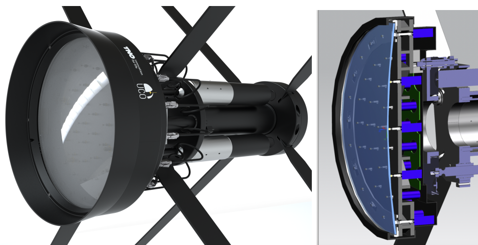
Figure 7.7 The APF ASM secondary assembly model as designed by TNO.
