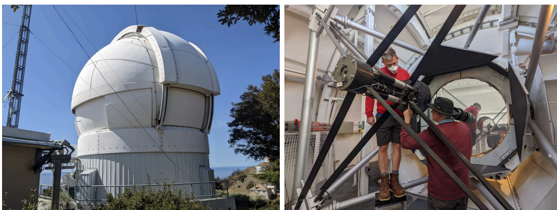
Figure 7.5 The 2.4m Automated Planet Finder Telescope ( Left ) The outside of the APF dome. ( Right ) An inspection of the current APF secondary mirror assembly.
