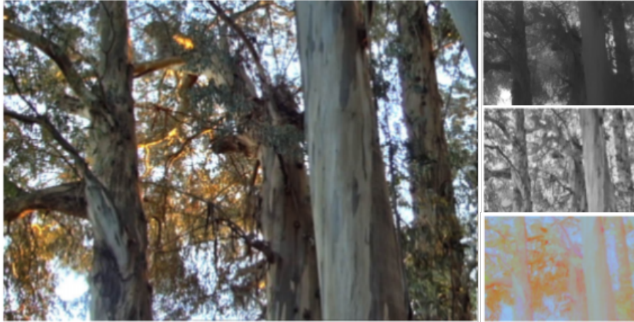
Figure 2.5: Results from [7]. The right images show the decomposition of the original HDR image. From top to bottom they are the Base, and Detail layers as well as the Color. The left shows the final image.
