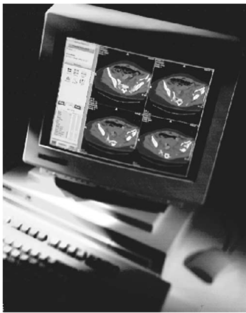
PACS workstation 1980's - single display unit running on a UNIX workstation
