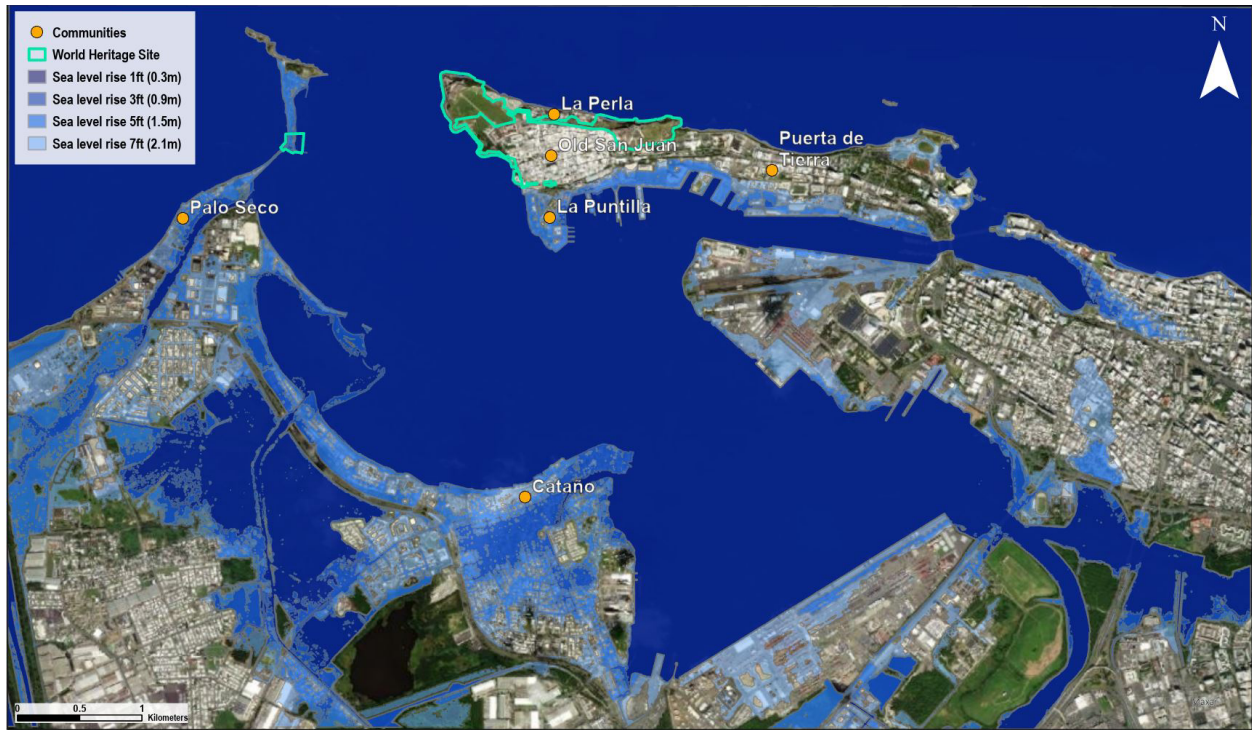
Figure 2: areas flooded around San Juan Bay under different sea level rise scenarios (map produced in ArcGIS Pro with data from NOAA’s Sea Level Rise Viewer online tool).
