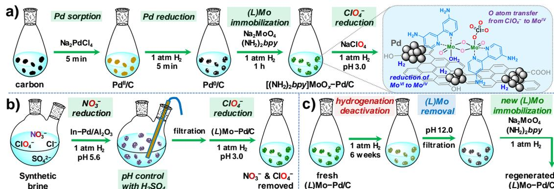
**Figure 5.1** Illustrated experimental procedures for (a) preparation of (L)Mo–Pd/C with adjustable Pd and Mo contents, (b) sequential reduction of  $\text{NO}_3^-$  by In–Pd/ $\text{Al}_2\text{O}_3$  and  $\text{ClO}_4^-$  by (L)Mo–Pd/C, and (c) hydrogenation deactivation and regeneration of (L)Mo–Pd/C.
