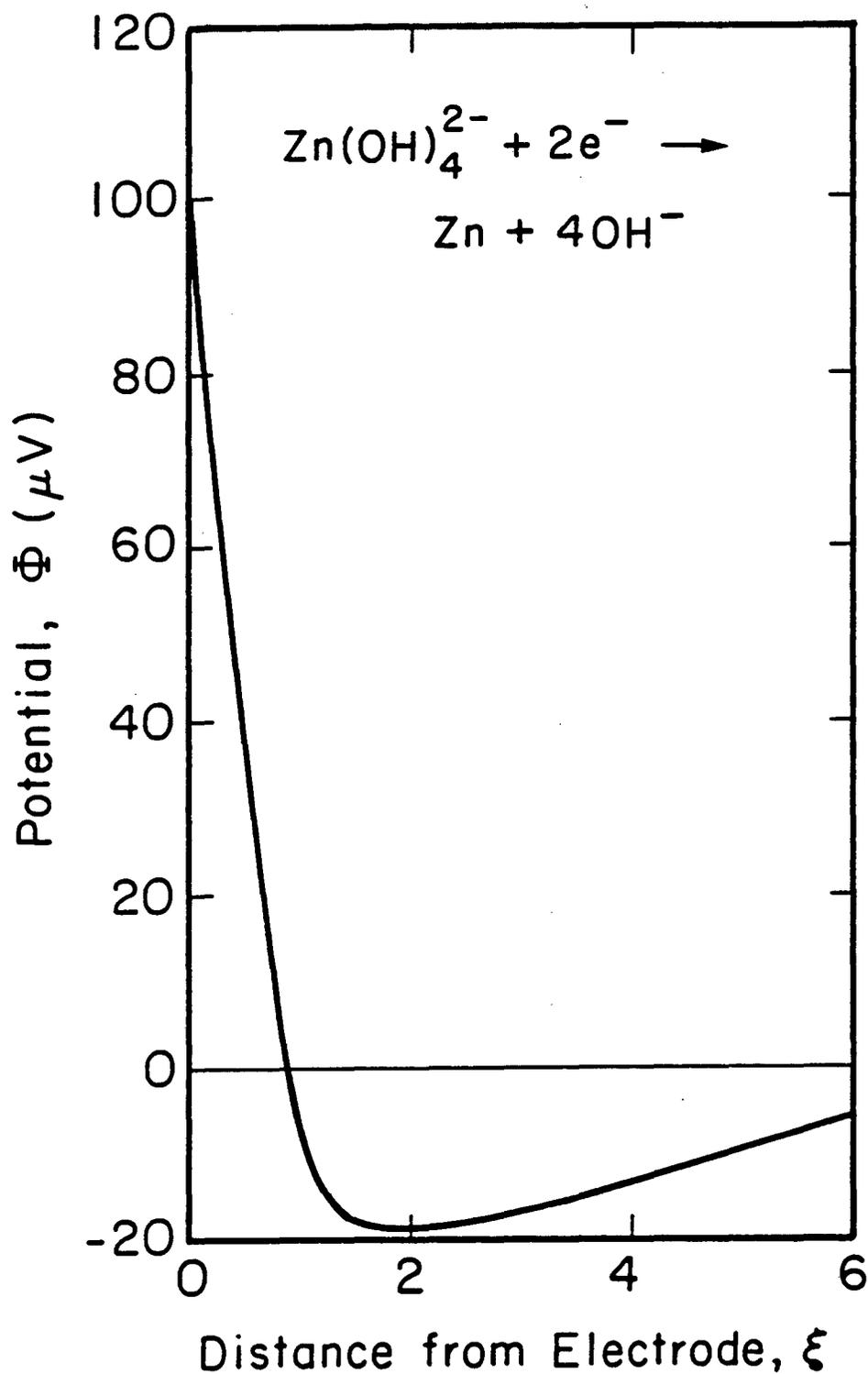
Figure 4. Potential profile as a function of the dimensionless distance  $\xi$  from the rotating disk ( $\Omega = 1600$  rpm) for zincate reduction at the limiting current in an excess of KOH supporting electrolyte ( $c_A = 19.8$  mol/cm<sup>3</sup> KOH and  $c_B = 0.1$  mol/cm<sup>3</sup> K<sub>2</sub>Zn(OH)<sub>4</sub>).
