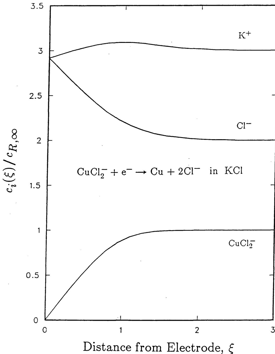
**Figure 2.** Concentration profiles for the cathodic reduction of  $CuCl_2^-$  at the limiting current in an excess of KCl supporting electrolyte. A constant has been added to the concentration ratios for the  $K^+$  and  $Cl^-$  ions so that they can be plotted together with the limiting reactant but otherwise undistorted.
