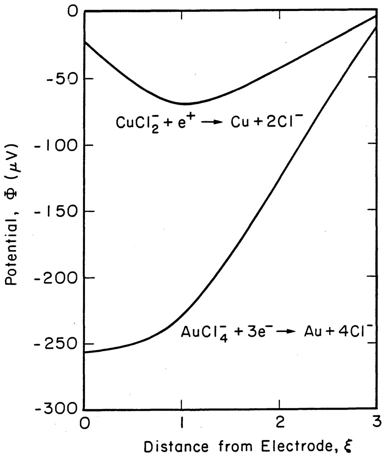
**Figure 3.** Potential profiles for gold and copper deposition at the limiting current in an excess of potassium chloride ( $r = 0.99$ ),  $c_A = 0.02 \text{ mol/cm}^3 \text{ KCl}$ ,  $c_B = 2.02 \times 10^{-4} \text{ mol/cm}^3 \text{ KMCl}_2$ , and  $\Omega = 1600 \text{ rpm}$ .
