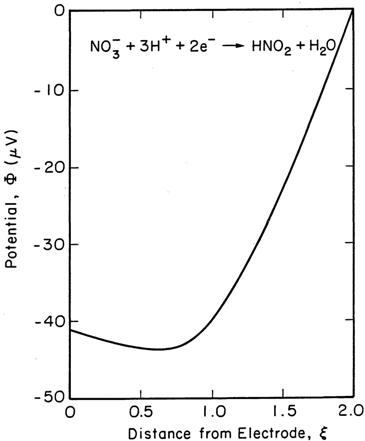
**Figure 5.** Potential profiles for nitrate reduction at the limiting current in an excess of  $\text{Ni}(\text{NO}_3)_2$  ( $r = 0.999$ ),  $c_A = 2.56 \text{ mol/cm}^3$   $\text{Ni}(\text{NO}_3)_2$ ,  $c_B = 0.005 \text{ mol/cm}^3$   $\text{HNO}_3$ , and  $\Omega = 1600 \text{ rpm}$ .
