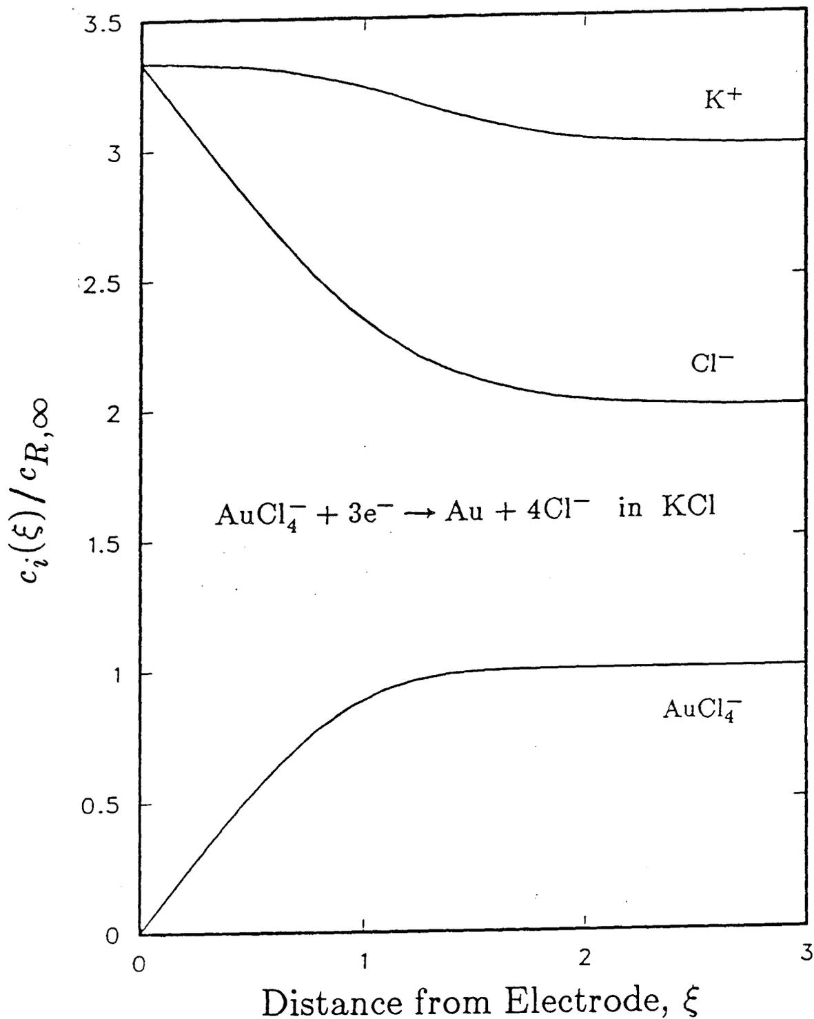
**Figure 1.** Concentration profiles for the cathodic reduction of  $\text{AuCl}_4^-$  at the limiting current in an excess of KCl supporting electrolyte. A constant has been added to the concentration ratios for the  $\text{K}^+$  and  $\text{Cl}^-$  ions so that they can be plotted together with the limiting reactant but otherwise undistorted.
