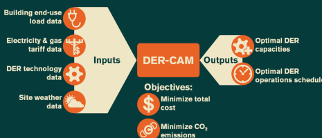
Figure 3: Diagram of major inputs, outputs and objectives in DER-CAM
