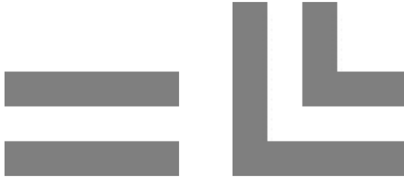
Figure 2.4: Two example patterns with the same minimum distance (50nm) studied in FEM analysis using COMSOL.
