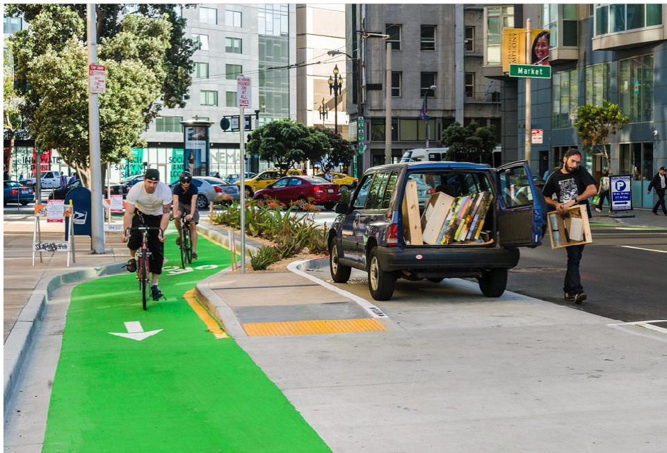
Figure 1.2. Protected bike lane and loading zone in a city street. Photo Courtesy of Flickr/Sergio Ruiz
