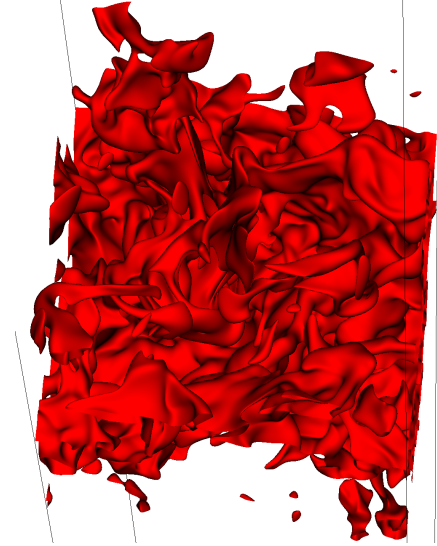
Figure 6. Isosurface (temperature of 1225K) for methane flame data set extracted using our algorithm. The isosurface consists of approximately 29.7 million triangles.
