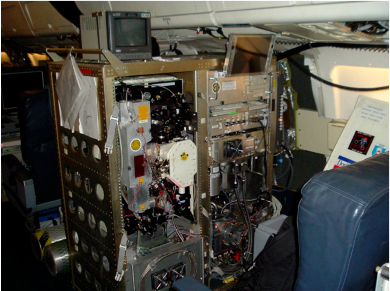
Figure 1.8: An extremely high precision spectroscopic NO 2 sensor mounted with an intake out the window of a DC8.
