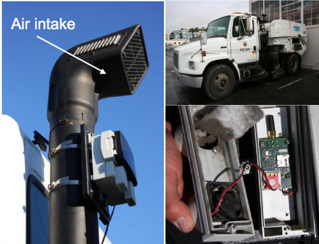
Figure 1.6: A sensing device mounted on a street sweeper in San Francisco as part of the Intel CommonSense project.
