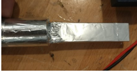
Figure 5.2: A photograph of the foil-wrapped PMT, waveguide, and scintillator.
