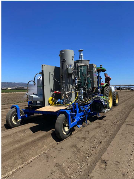
Figure 5: Clayton Steam applicator from Yuma, Arizona.
