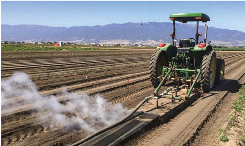
Figure 4: The bed shaper used as a steam applicator in 2020.
