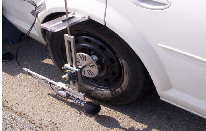
Figure 3: On-board sound intensity (OBSI) microphone setup.
