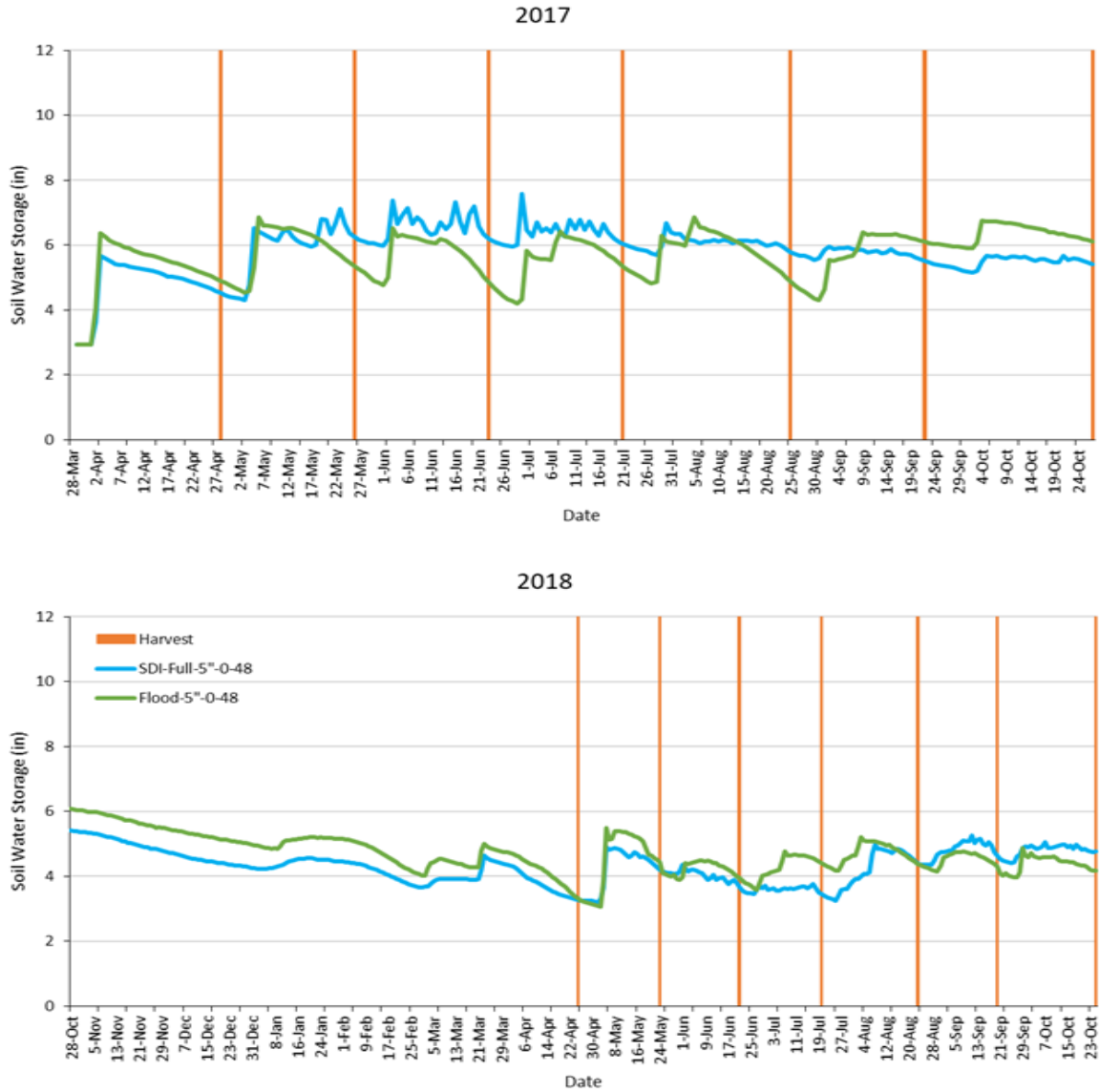
Figure 1.9. Soil water storage (inches) in top 120 cm for surface irrigation (Green line) and SDI (Blue Line) along with harvest dates (orange verticle bars) for the year 2017 and 2018.
