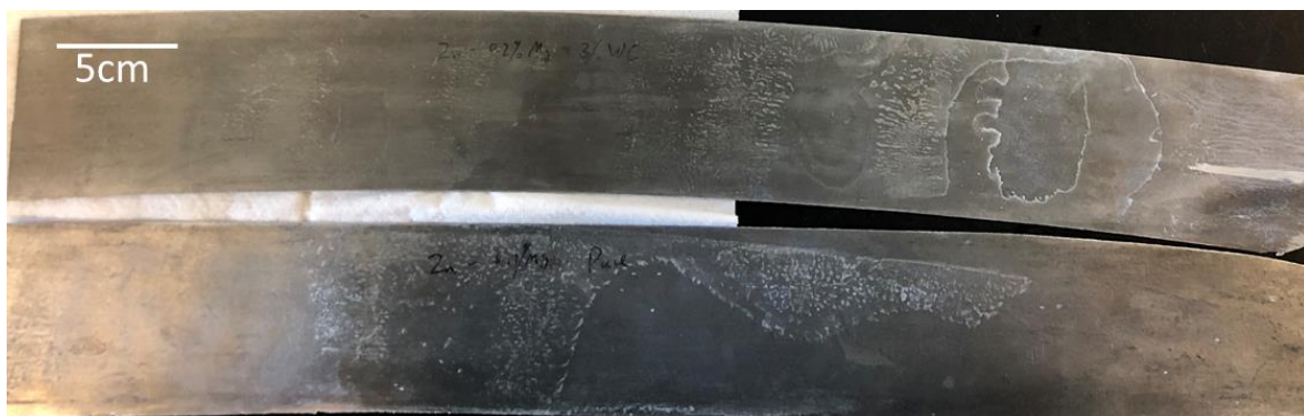
Figure 12 Hot-rolled Zn-WC thin sheets
