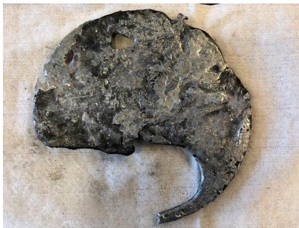
Figure 10 Failed cast sample
