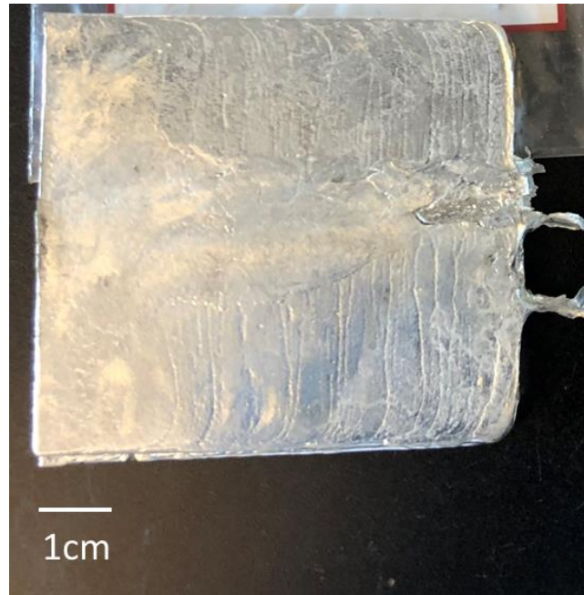
Figure 11 Zn-WC cast sample
