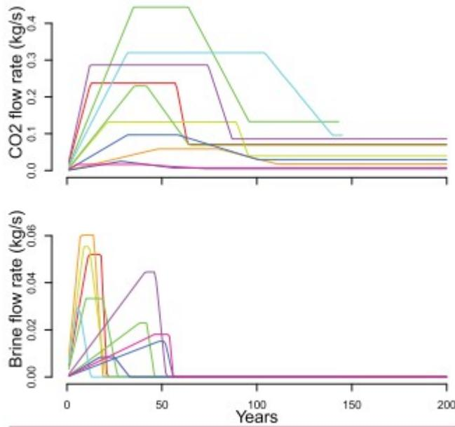
Figure 4. Subset of CO<sub>2</sub> and brine flow rate scenarios generated by the heuristic leak model in AIM
