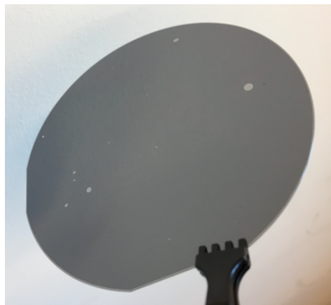
Figure 2.3.2 | Glass wafer (top side) bonded to silicon wafer (bottom side). Wafer size is 4 inch. The white dots are the bubbles generated from the wafer bonding process.
