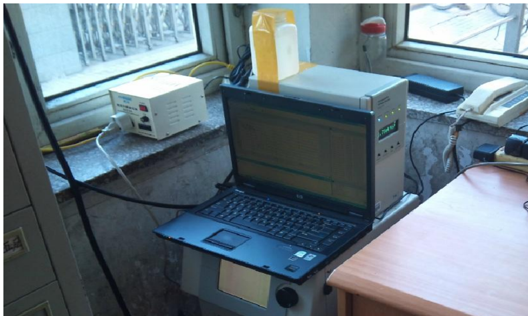
Figure 3: Roadside/Downwind site CPC indoor setup
