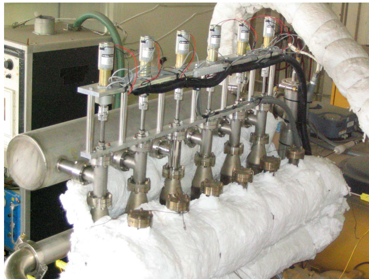
Figure 2.6: Dual manifold intake system implemented in the Caterpillar engine for HCCI combustion control. The figure shows the cold manifold, the hot manifold (insulated with white material), and the mixing valves actuated by servo motors (top of the picture ).
