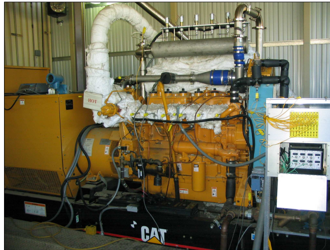
Figure 2.1: Engine used in HCCI experiments, 14.6 L, 6 cylinder natural gas engine setup for stationary power generation.
