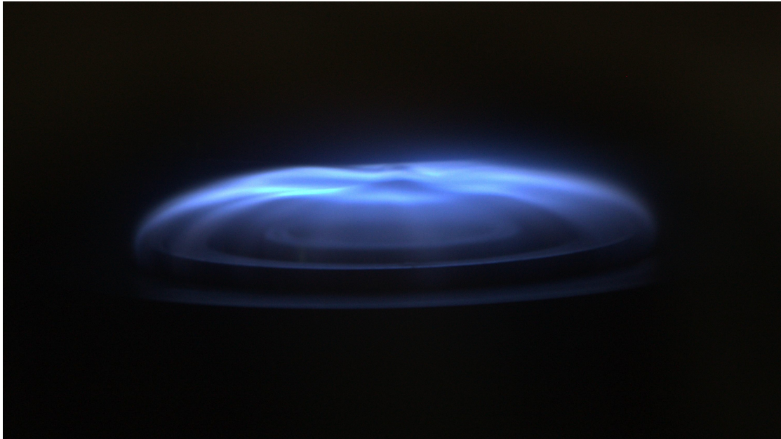
Figure 3.13: Photograph of a nonpremixed methane-air flame with a fuel mass fraction Y_{F,1} = 0.14 at 1.6 MPa displaying radial streaks.
