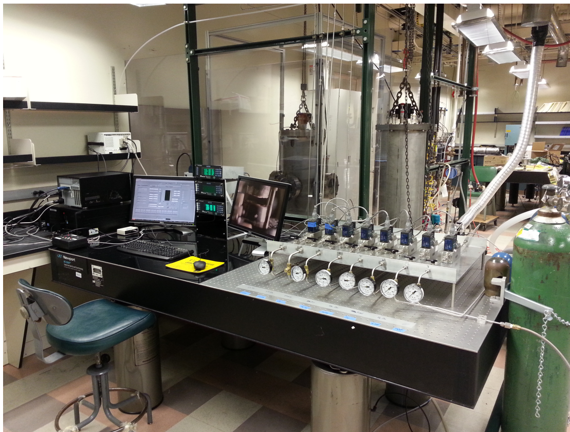
Figure B.7: Photograph of the HPCEF control station, showing the control and data acquisition unit (left) and the mass flow controller bench (right).
