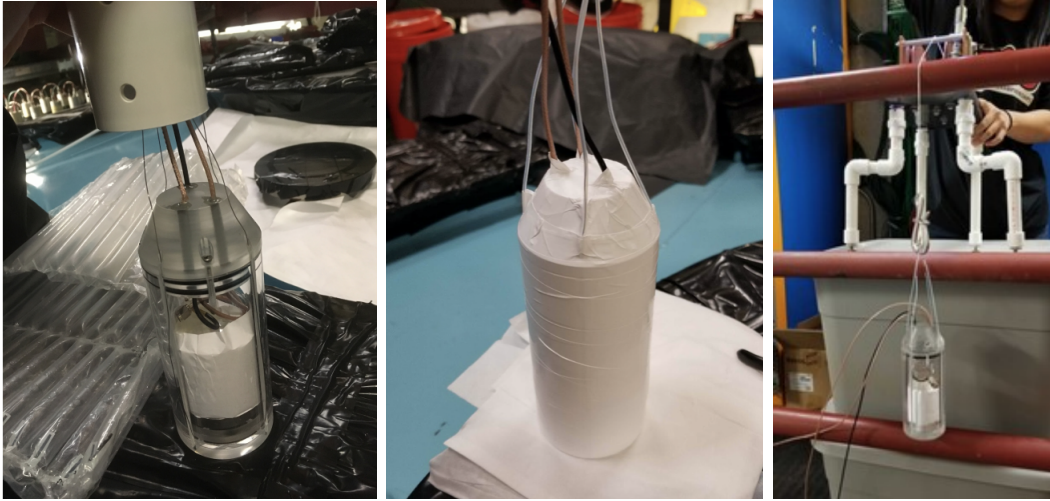
Figure 5.13: LEFT: AmBe source in acrylic housing. A deployment mechanism was being tested here. CENTER: AmBe source housing wrapped in teflon (PTFE) tape to maximize light collection. RIGHT: AmBe source deployment winch being tested. This was the method selected for deployment.
