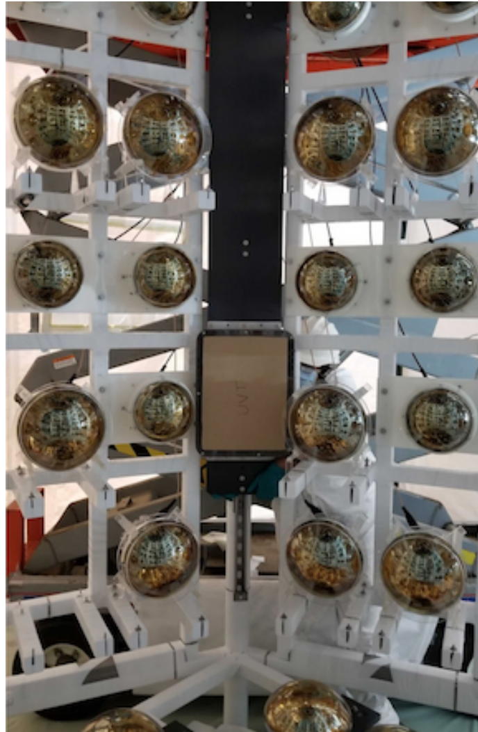
Figure 4.25: An empty LAPPD housing attached to a deployment panel. Testing of the deployment mechanism took place in a clean tent, before the octagonal inner structure was transported to ANNIE Hall. The panel slides along the rail via polypropylene sliders bolted to its back. All eight panels were tested to make certain that they slid down the rails smoothly. Sliders that did not go down a track smoothly naturally had pieces of polypropylene shaved off by the track. An ANNIE collaborator can be seen behind the inner structure holding the deployment panel.
