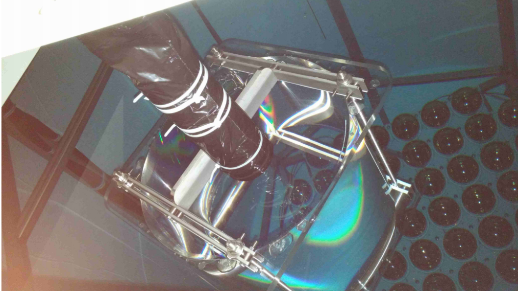
Figure 3.1: The Neutron Capture Volume (NCV) is an acrylic vessel filled with EJ-335, a mixture of liquid scintillator and gadolinium. A PMT coupled to the NCV is wrapped in black to prevent light generated in the tank from triggering the data acquisition system. The array of PMTs at the bottom of the Phase I detector can be seen facing upward in this image.
