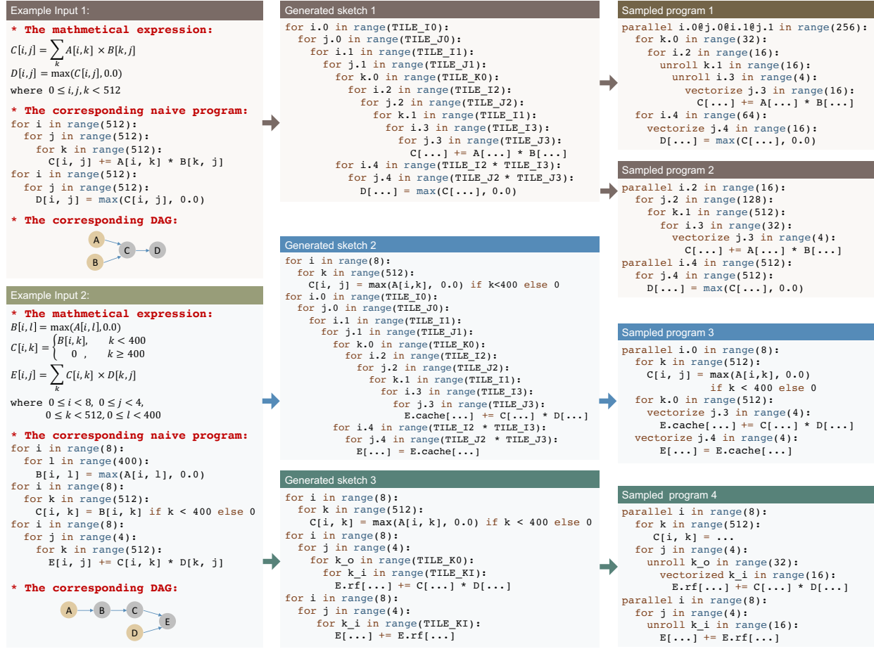
Figure 3.5: Examples of generated sketches and sampled programs. This figure shows two example inputs, three generated sketches and four sampled programs. The code example is pseudo code in a python-like syntax.
