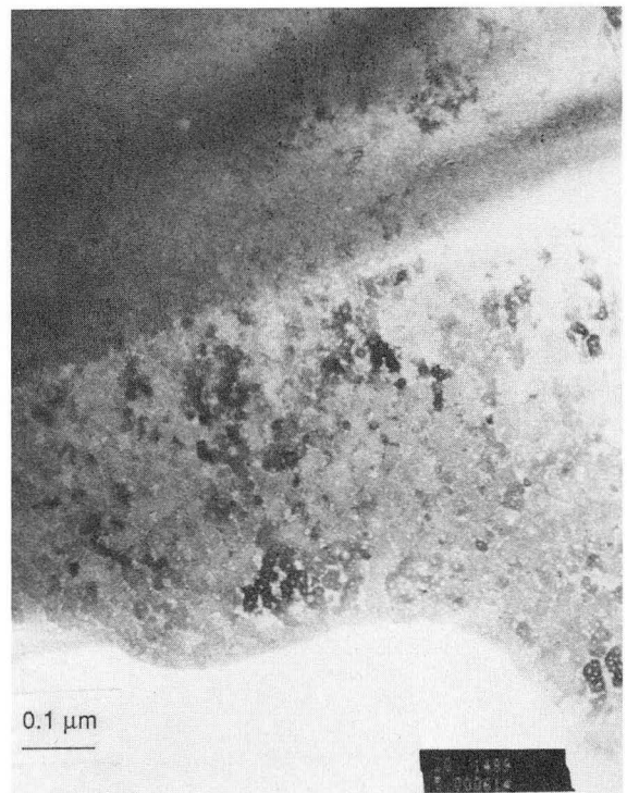
Figure 2 A TEM plan-view micrograph of Zn-diffused InP showing the presence of a large concentration of precipitates of different phases. Two phases of Zn_3P_2 and Zn microcrystals were identified by the Bragg reflection technique. XBB 903-2668
