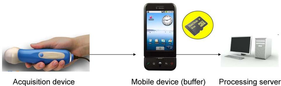
**Figure 2. Data Storage Mechanism.** The raw data flowing from the mobile device which acts as a storage device. Once a connection is available, the data is being transferred to the server for processing.
