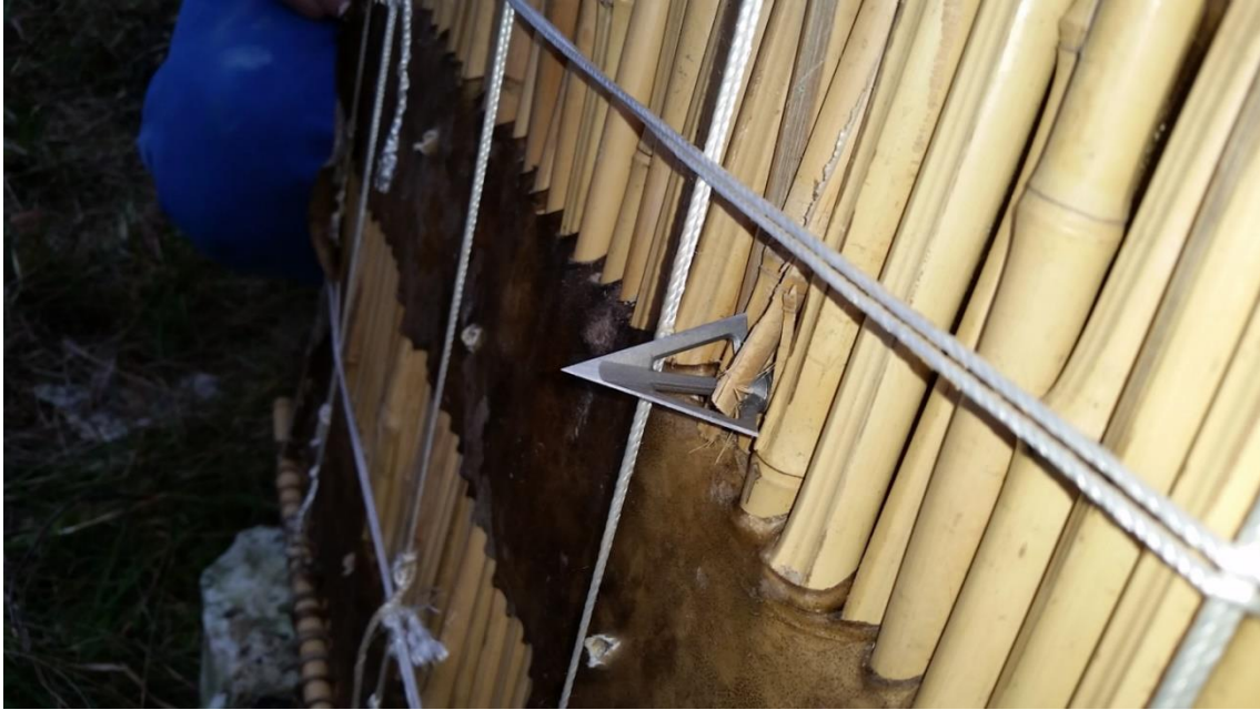
Fig. 4.6 – Broadhead penetration of reconstructed gerrhon
