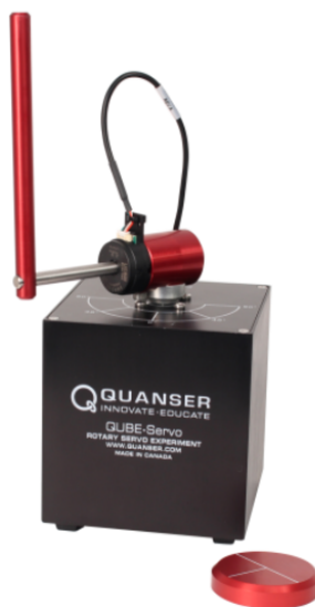
Figure 4.23: Quanser-Servo2 inverted pendulum system hardware [1].
