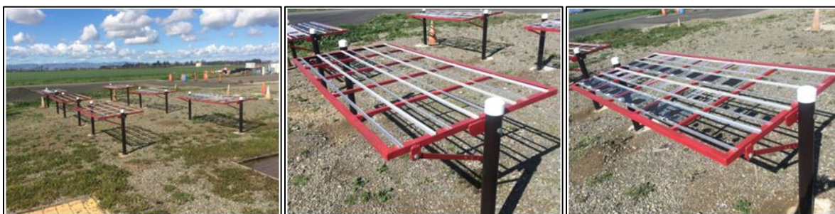
Figure 4.2: Six aging racks (left), an unloaded aging rack (center), and aging rack loaded with glass plates (right).
