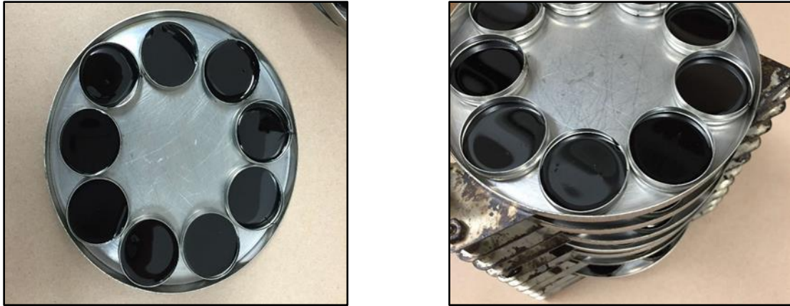
Figure 4.4: Modified PAV loading - small tin loaded in standard PAV pan (left), loaded tins put in PAV frame (right).
