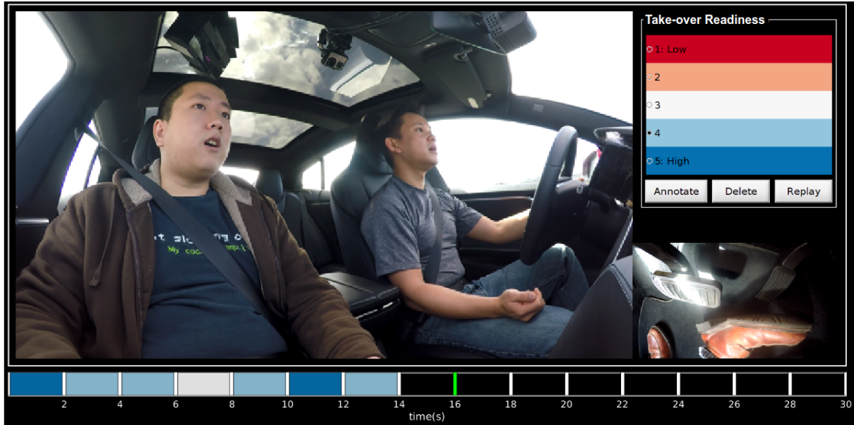
Figure 6.3. Interface for collecting ratings: The raters observe video feed from the pose and foot cameras and assign a rating for each 2 second segment of video.
