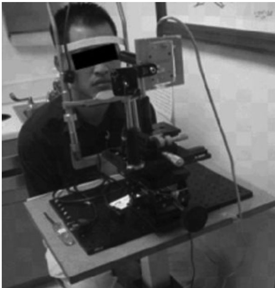
Figure 3. This figure displays the optical apparatus used for human tear film thickness measurements. The laser and the camera assembly were placed on mechanical stages equipped with X-Y-Z movement. The imaging system is mounted onto a track for scanning purposes. Subjects placed their head on the chin-rest and maintained a constant focal length with respect to the camera assembly. Data were streamed to a computer for further computational analysis.
