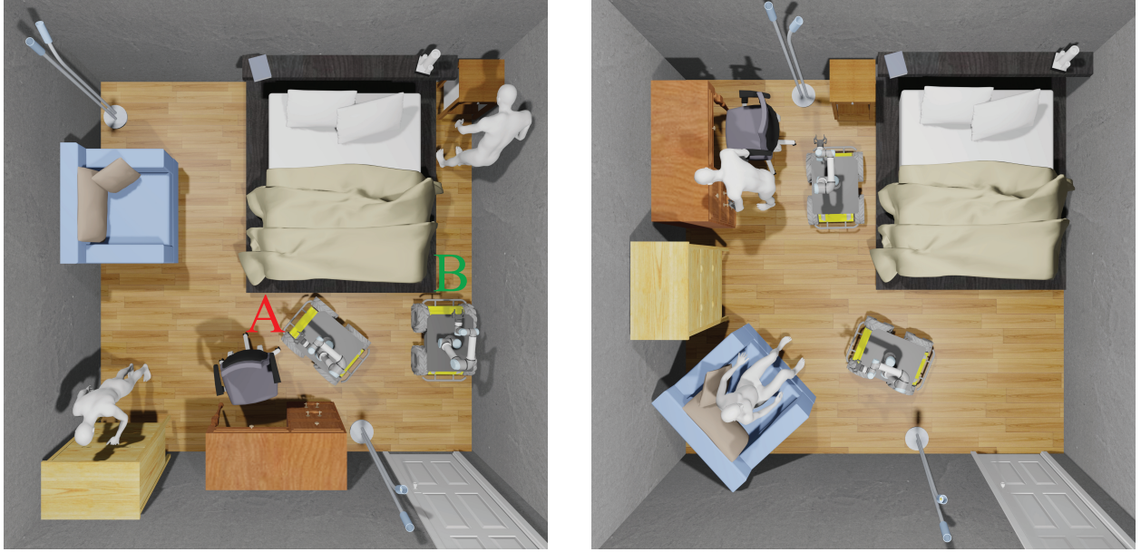
Figure 4.1: A human-activity layout (left) can exclude a mobile manipulator at the passages marked A and B even though people can use the room. The published rearranged layout (right) creates traversal and approach space while preserving human functional relations. Reproduced from the published co-activity study (Wang et al., 2023). © 2023 IEEE.
