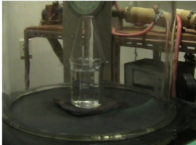
FIGURE 5. Torricelli setup inside the receiver (glass jar) of a vacuum pump, consisting of a beaker nearly full of water, and an initial column of water in an inverted glass tube held in position by tape. The vacuum pump with a pressure gauge is seen in the background.
