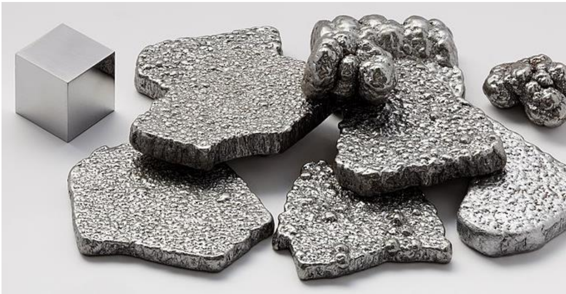
Figure 2-1. Pure iron chips, electrolytically refined and high purity (6N) 1 cm 3 iron cube [1].
