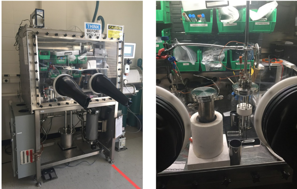
Fig. 4. (a) Argon glovebox (LC Technology Solutions, Inc.). (b) Electrochemical cell in glovebox.
