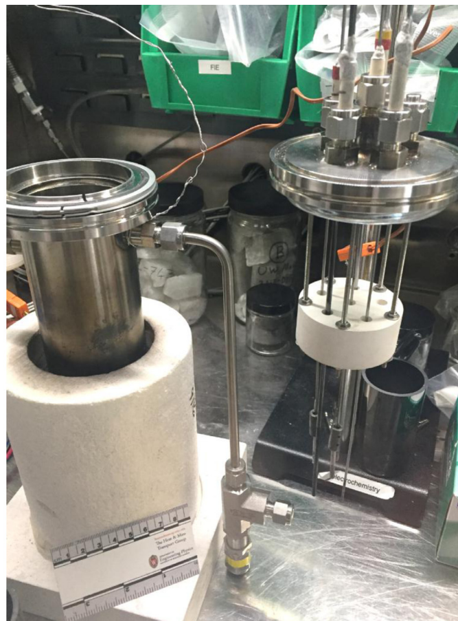
Fig. 1. (a) Cross-section view of electrochemical cell. (1) Thermocouple, (2) thermowell, (3) Swagelok tube fittings (5x), (4) top lid, (5) centering ring, (6) alumina tube, (7) gas control tube fittings, (8) cell body, (9) heat shield, (10) furnace, (11) crucible, (12) electrode connector, (13) electrode sleeve, (14) centering disk, (15) furnace base, (16) active cooling region. (b) Photograph of electrochemical cell with top cell flange assembly removed from cell body.
