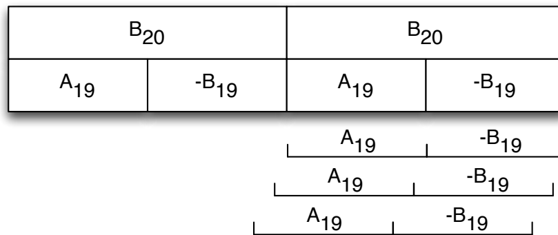
Figure 6.1: Extracting complementary pairs from concatenated B_{20} sequences
